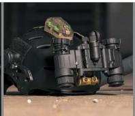
The AGM FoxBat night vision bi-ocular is the perfect tool for mid-range and long-range observation. The FoxBat combines a single high quality image intensifier tube with an image beam splitter and double eyepiece, making it applicable for long viewing sessions. The FoxBat is packed with features such as digital controls, and a proximity sensor for automatic shut off in varying light conditions. This night vision bi-ocular is the ideal choice for security and recreational use.
